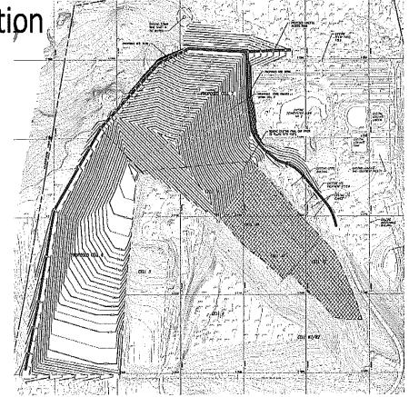
Mr. Beebe referred to slide number two. He stated that this was essentially the base liner layout of the landfill and the grading for the base liner and that it also showed access roads. He noted that this also shows where the M.S.E Berms will be placed.
